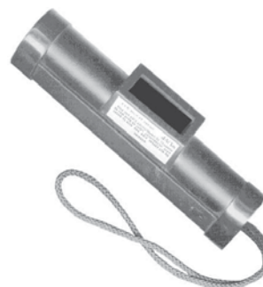
951.199 UV-Lamp for Float Glass An invaluable aid in determining the tin side of float glass. Battery powered.
